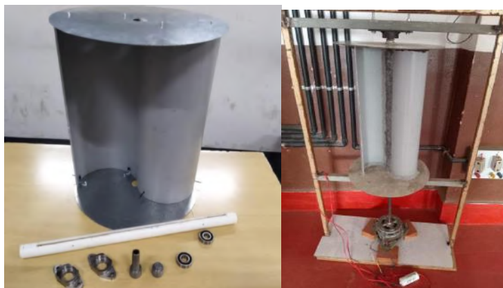
Fig. 6. Hardware architecture- Prototype of VAWT
