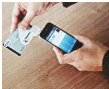
A user demonstrates how Square works: The card reader fits into the phone's audio jack. The vendor slides the card through the magnetic reader, the card holder provides a signature on the phone's touchscreen, and the transaction is processed in less than 60 seconds [if the wireless connection is good].
