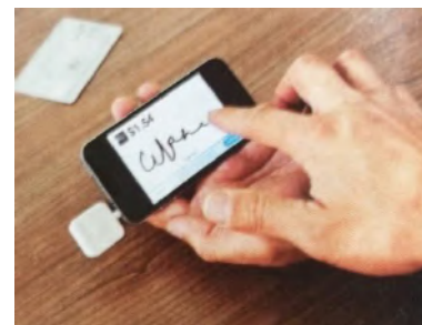
A user demonstrates how Square works: The card reader fits into the phone's audio jack. The vendor slides the card through the magnetic reader, the card holder provides a signature on the phone's touchscreen, and the transaction is processed in less than 60 seconds [if the wireless connection is good].
