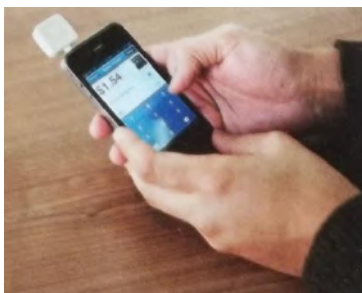
A user demonstrates how Square works: The card reader fits into the phone's audio jack. The vendor slides the card through the magnetic reader, the card holder provides a signature on the phone's touchscreen, and the transaction is processed in less than 60 seconds [if the wireless connection is good].
