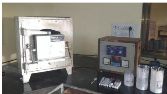
FIGURE 1. Sample being calcinated at 1200^\circ\text{C} in a furnace
