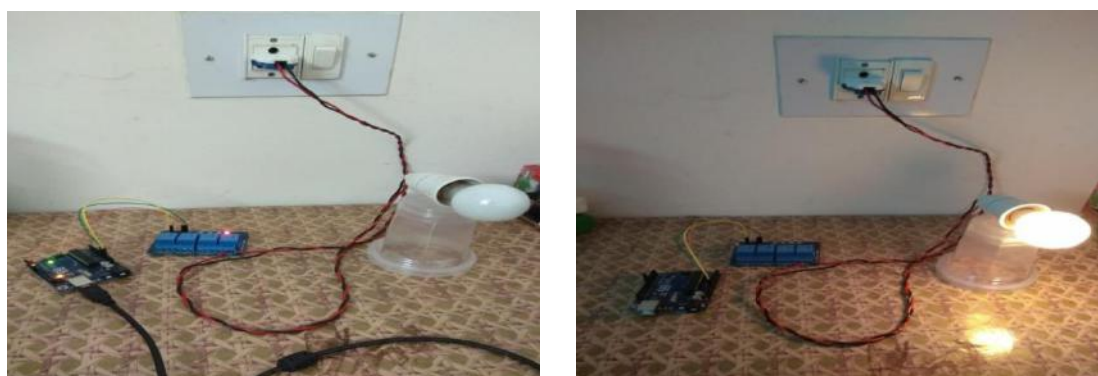
Fig 1.9 Output of relay controlled AC devices
