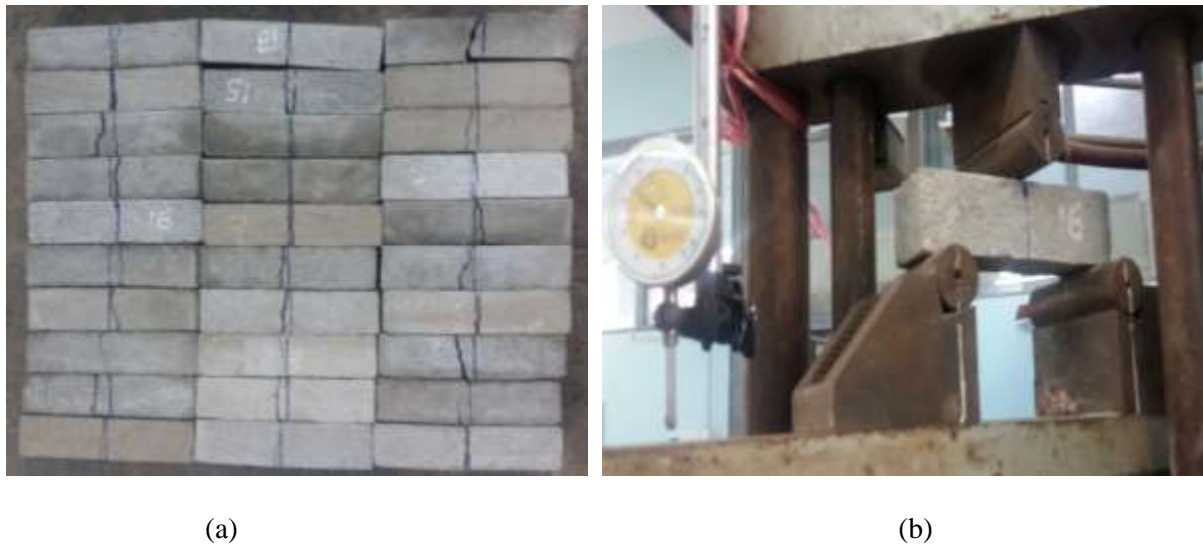
Figure 4: (a) Flexural strength test specimens 40mm x 40mm x 160mm size (b) Flexural strength test of mortar beam Trebel Universal Testing Machine-40KN machine
