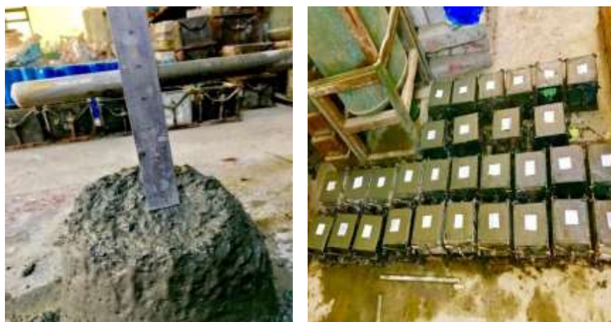
Figure 3: Slump Test and Cube Casting
