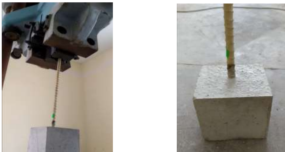
Figure 2. The process of testing the bonding of glass composite fittings with concrete .
