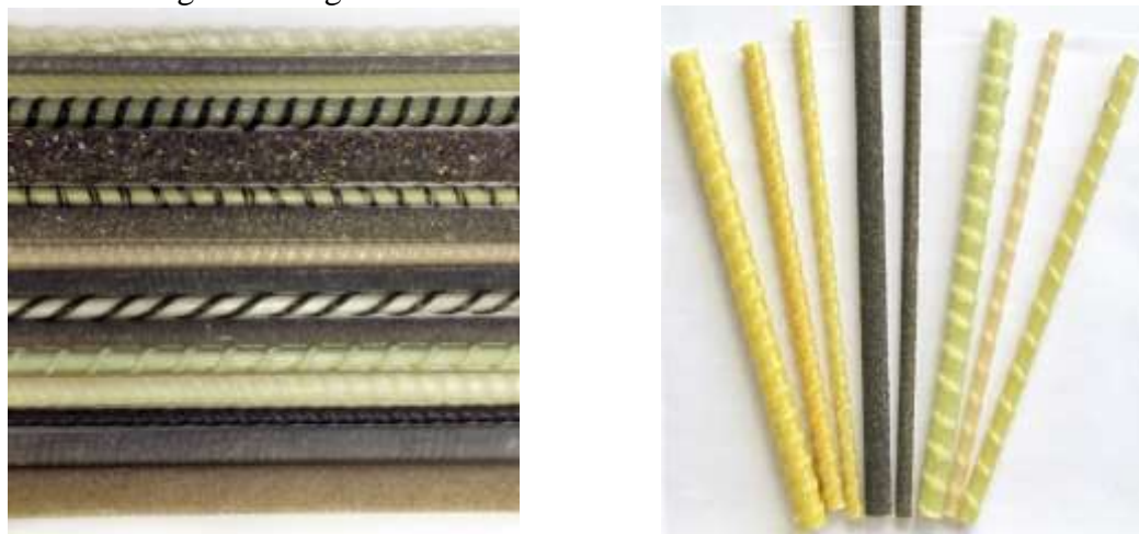
Figure 1. Basic types of surface part of glass composite fittings with artificial irregularities and sand coating.
