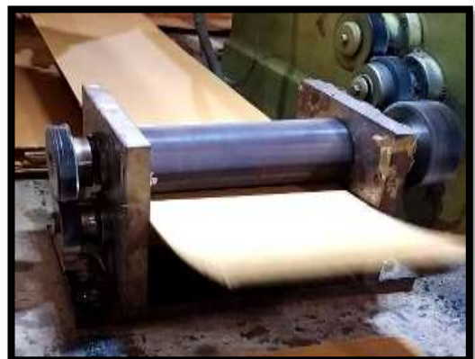
Fig 5.3: Corrugated board fed into the knurling tool
