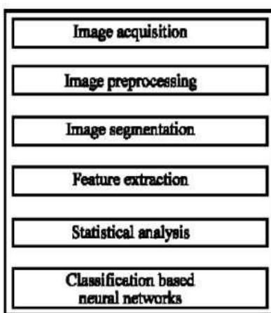
Figure. 2. Basic Procedure of Leaf Disease Detection System
