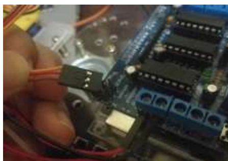
Figure 17. Wire up the Servo Motor to Motor Shield (Servo _ port 2)
