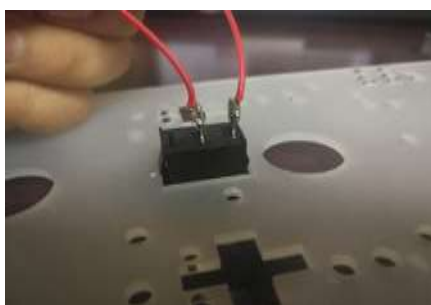
Figure 13. Soldering the ON/OFF Switch
