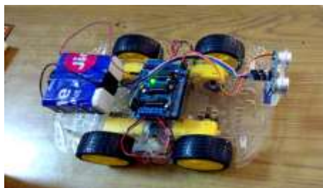
Figure 14. The hardware model depicting my project model (Obstacle Avoiding Robot).
