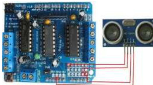
Figure 16. Block Diagram of connect ultrasonic sensor Pins to the Motor Shield.
