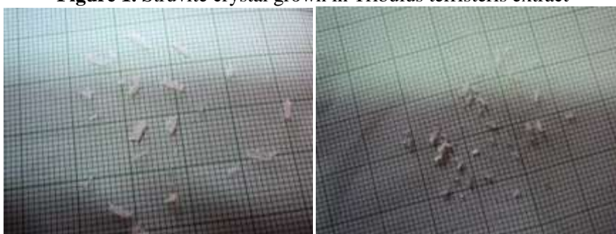
Figure 1. Struvite crystal grown in Tribulus terrestris extract
