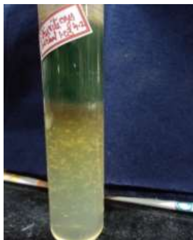
Figure 1. Struvite crystal grown in Tribulus terrestris extract
