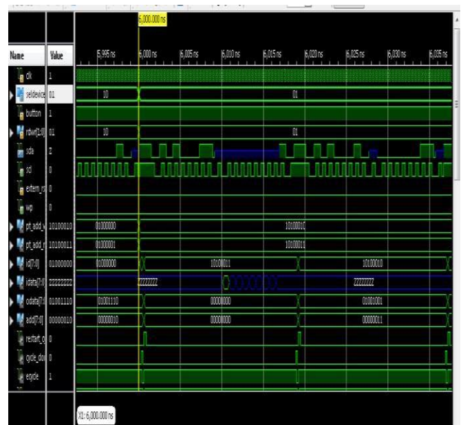
Figure 5.: Shows register address change for write operation on DS1307 IC
