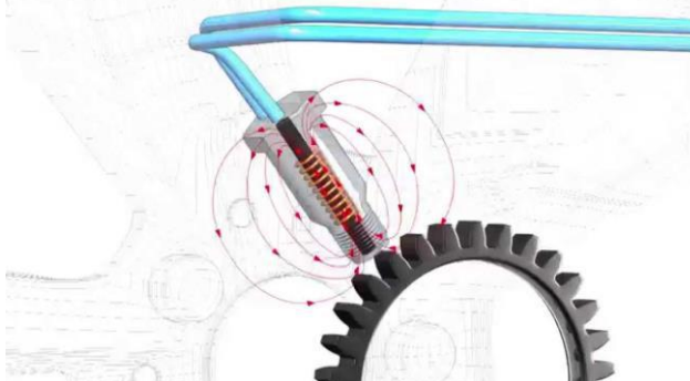
Fig 6. Wheel speed sensor
