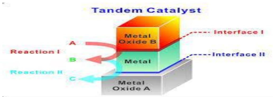
Fig:-1 Image of mixed metal oxide nanoparticles tandem catalyst.
