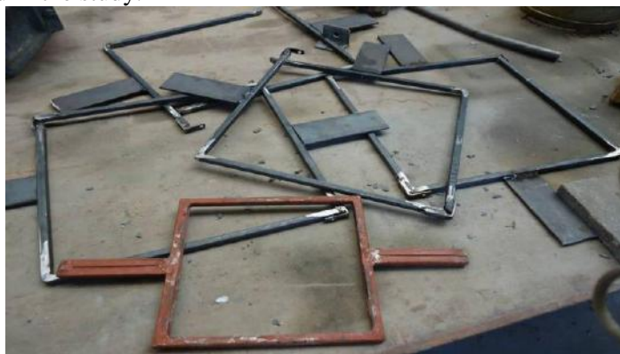
Fig 1.3 Moulds for tiles casting
