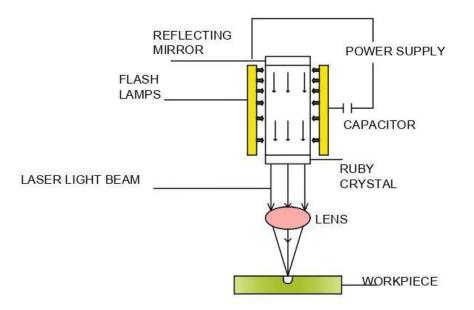
As seen in the picture, the laser crystal is in the form of a cylinder whose flat actuator head is placed in a flash lamp coil of about 1000 watts. A flash with high intensity white light is emitted from the crystal. The crystal is excited and emits a laser light beam which is focused onto the surface of the workpiece using a lens. The laser light beam produced is
