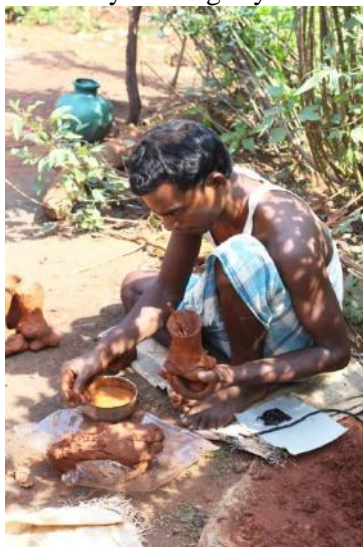
Mould making process of Dokra casting ( Dhenkanal, Orissa) (Baral and Rashitha)
