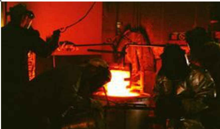
The workers at Schaefer Foundry in Arlington, TX, carefully lift up the crucible, containing the molten bronze, out of its heating furnace. Photograph by Elizabeth Loggins.
