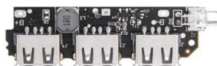
Fig. 2.6: Power Bank Board Managing Charging and Discharging of the Power Bank.
