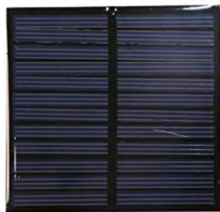
Fig. 2.1: Mini Solar Panel Used in the Solar Power Bank Prototype.
