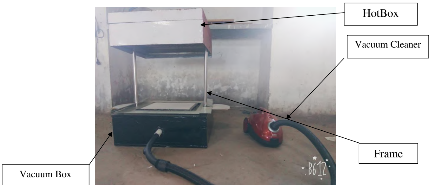
Figure 6.2 Vacuum Operated Plastic Molding Machine
