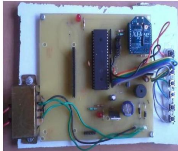
Fig.2.2: Circuit of Transmitter Module
