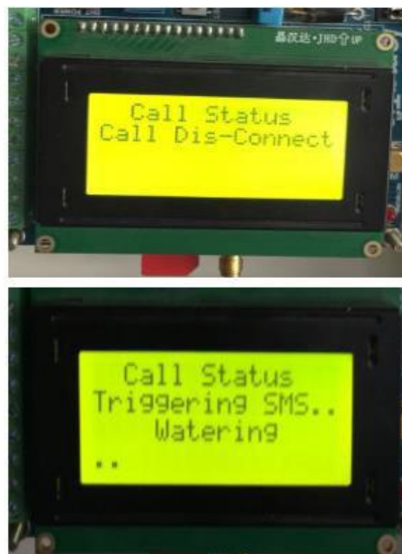
Fig. Start motor then Disconnect call Triggering SMS
