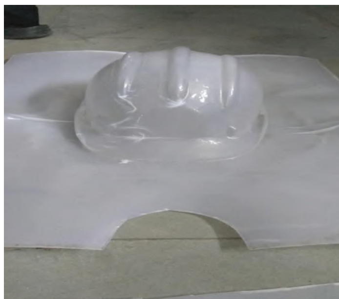
Figure 6.3 Workshop Helmet Created on VOPMM
